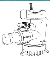
The SPX Johnson Pump Marine submersible pumps can handle most of the bilge pump applications. Heavy duty motors with stainless steal (SS2343) shaft and tough thermoplastic bodies provide for a long pump life. With an automatic switch installed, the pump automatically comes on when there is water in the bilge and shuts off when it is dry. Submersible bilge pumps are not self-priming and must be installed in the deepest part of the bilge.
